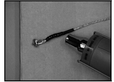
Step 3: Shrink WireWraps with a heat gun
